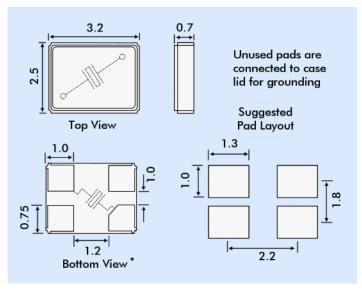
\* Note: These parts may be supplied with the chamfered pad in different positions. However, the crystal connection is always as shown above.
